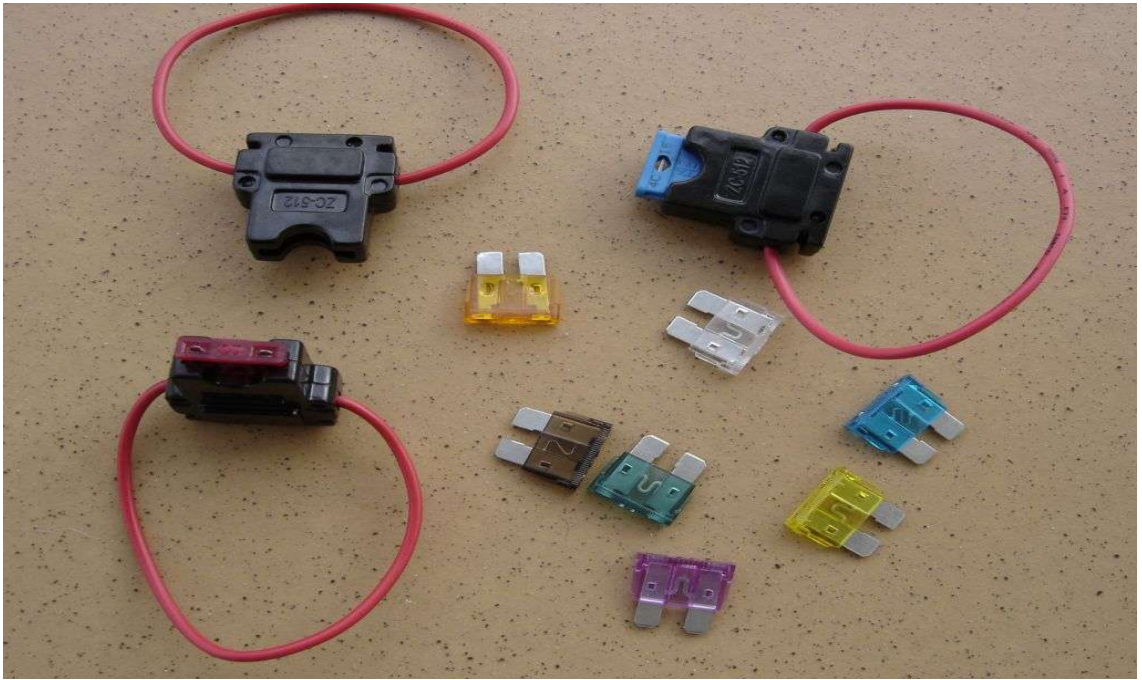
Here are typical blade fuse holders and fuses, each colour represents a value. The red lead just gets cut and joined to the wires being run.
