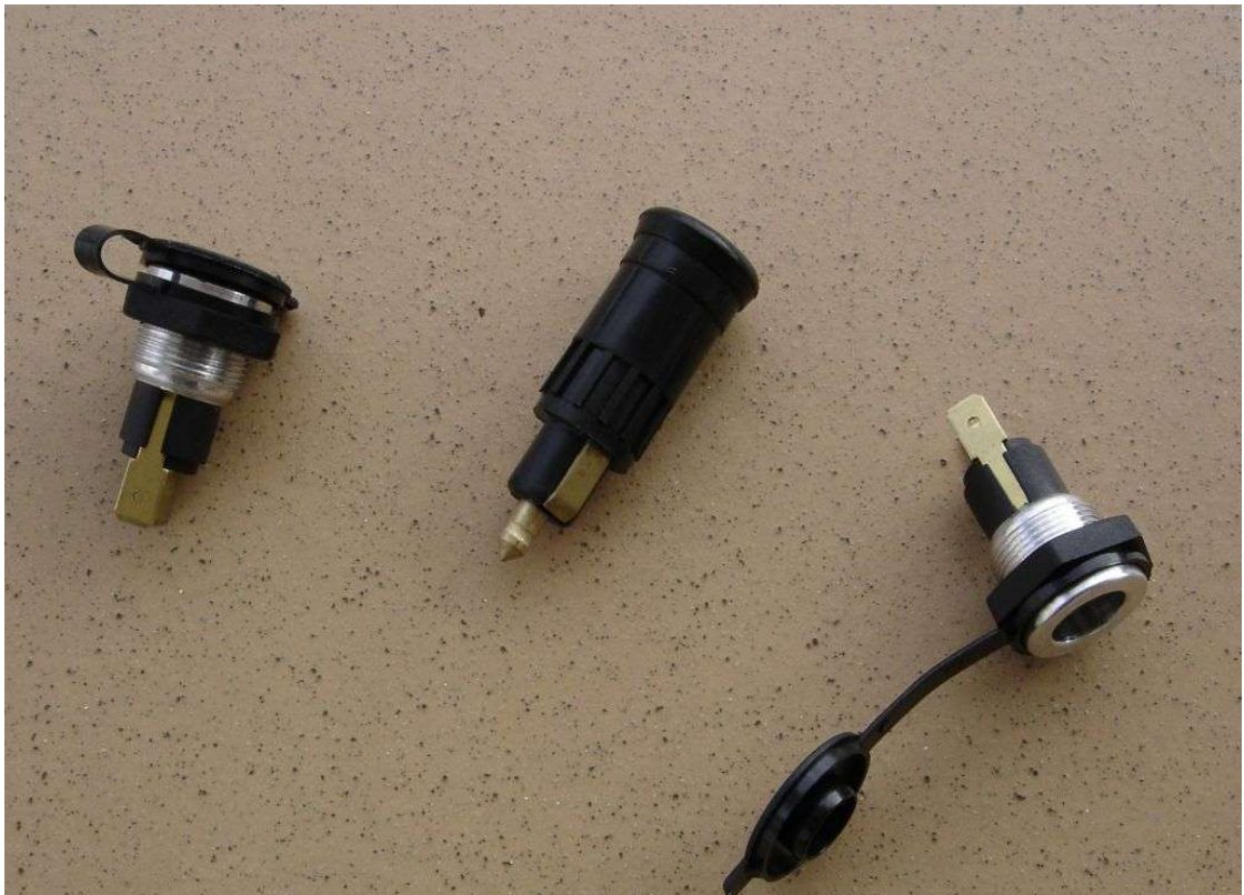
Here you have a typical 12volt weatherproof and robust socket and plug. These can be used to drive accessories and fitted in a convenient spot or even double up as you battery tender socket. An adapter to plug a cigarette lighter type socket can easily be made up as well, using the make plug and a short wire with female cigarette type socket.
